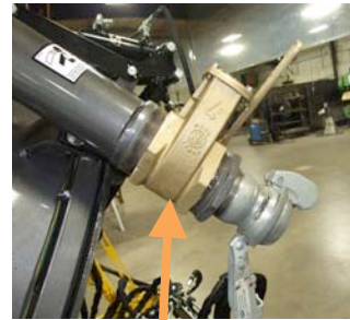
Suction Valve Lever up – Closed Lever down - Open
